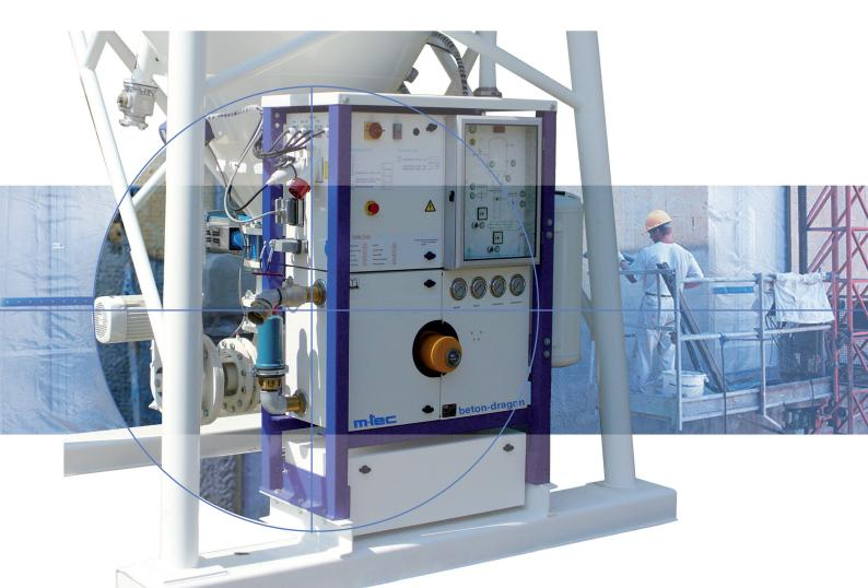
The beton-dragon-II was specially designed for the requirements when processing readymixed dry spraying mortar with a granularity of up to 4 mm and dry spraying concrete with a granularity of 4 - 8mm. This makes it ideal for new buildings and for repairing structural engineering projects from building construction and civil engineering to tunnelling.
