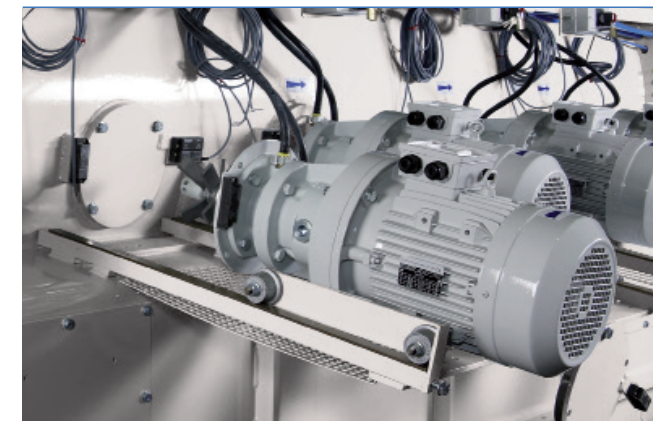
Option: agitator quick change system
